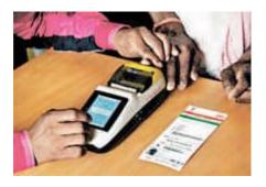
This device will be based on a mobile phone connection and would be made available to every Bank Mitra / Business Correspondent. Customers would have to get their identity authenticated and withdraw or put money into their bank accounts. The basic transaction types to be supported by micro ATM are Deposit, Withdrawal, Fund transfer and Balance enquiry. Micro-ATM offers one of the most promising options for providing financial services to the unbanked population.
